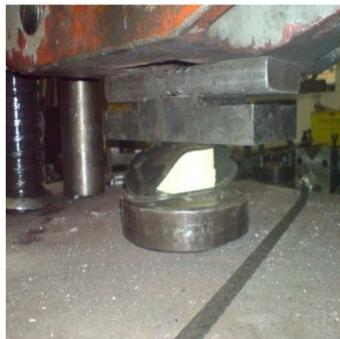
Fig. 6. Sulfur concrete compression test.
