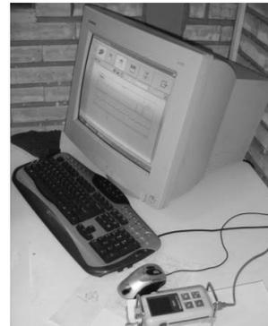
**Fig. 3.** The roughness tester model MarSurf TS1.
